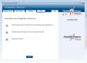
You have already completed steps 1 and 2; click on *Continue* at the bottom. A count-down now starts, while Terminal waits for the **GPS II** to switch to PC control; this screen now appears:
