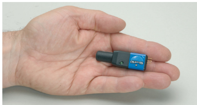
As can be seen, the sensor is particularly compact, notable is the green LED, which indicates if the sensor is hunting for satellites or is in full operation
