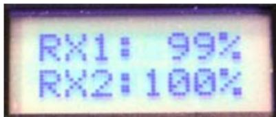
**Important!** The percentage figure after RX 1 and RX 2 always indicates a proportion of the duration of the last flight.
