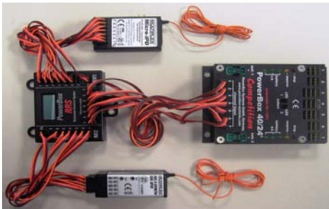
The photo below shows the method of connecting the system using a **PowerBox Evolution**. Seven channels of the Futaba G3 receiver are connected to the **RRS** module, plus the fail-safe channel. Since the **PowerBox Evolution** only caters for five remotely accessed channels, there are two vacant sockets on the **RRS** module to which two more servos can be connected. All the remaining channels of the Futaba G3 receiver could also be used directly at the receiver.
