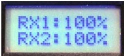
If this display appears, the receivers 1 and 2 are both working correctly, both are exhibiting 100% reception.
