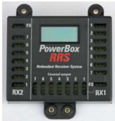
You must connect one channel to the fail-safe channel (FS socket) as for receiver 1, and this channel must be programmed to fail-safe at the transmitter.
