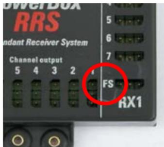
You will find the “Fail-Safe” sockets located close to the seven channel inputs for both receivers, but slightly apart from them; these sockets are marked “FS” on the **RRS** module. This socket should be connected to one receiver channel which you have programmed to fail-safe at the transmitter.
