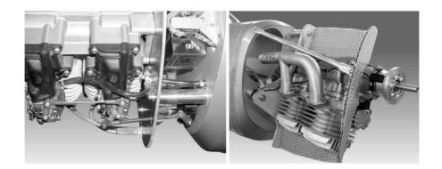
It is absolutely vital to ensure a tension free mounting of the engine. The surface that the engine is mounted on must be on an even plane (i.e., a flat and level surface) so that there is no strain on the engine itself. Again, this is a vital and critical requirement to avoid distorting the crank case, ruining the engine, and voiding your warranty.
