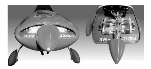
It is absolutely vital to ensure a tension free mounting of the engine. The surface that the engine is mounted on must be on an even plane (i.e., a flat and level surface) so that there is no strain on the engine itself. Again, this is a vital and critical requirement to avoid distorting the crank case, ruining the engine, and voiding your warranty.
