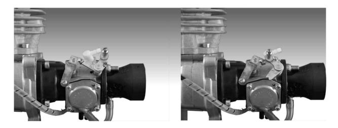
Note: The use of a soft pushrod for the throttle (plastic or nyrod) is not recommended. Use a metal or carbon fiber pushrod with a plastic ball joint or plastic clevis at each end. This will keep your RPM much more consistent and accurate around idle where it really counts.
