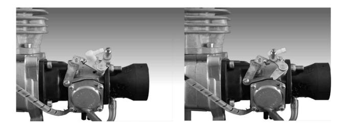
Note: The use of a soft pushrod for the throttle (plastic or nyrod) is not recommended. Use a metal or carbon fiber pushrod with a plastic ball joint or plastic clevis at each end. This will keep your RPM much more consistent and accurate around idle where it really counts.
