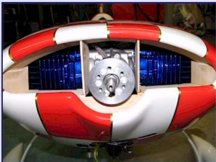
Front Baffle Made From 1/8" Balsa
