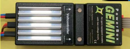
third servo lead is connected to the receiver output which controls the gyro or the gyro servo. At the other end of the Gemini is the red socket for the sensor switch, and adjacent to that is the socket for the gyro. At that point the gyro signal from the receiver is present, together with a second voltage level of 5.3 Volts.
