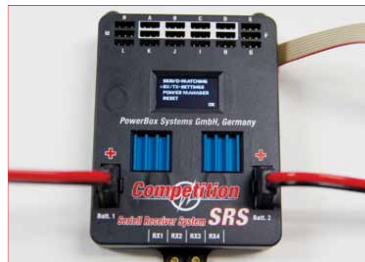
Entering this function will let you adjust the settings for both Rx and Tx. This is an intuitive process; however, PowerBox's instruction manual is one of the best I've ever used.
