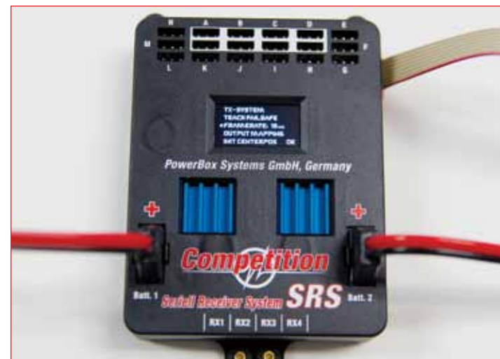
Here I've set the frame rate to 18 ms. From this screen you can also pick the type of transmitter you'll be using, such as Spektrum/JR, Multiplex, Futaba or Jeti.
