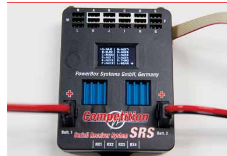
You can do output mapping to determine what port controls what function. You can also adjust servo travels, end points, travel volumes and centering.
