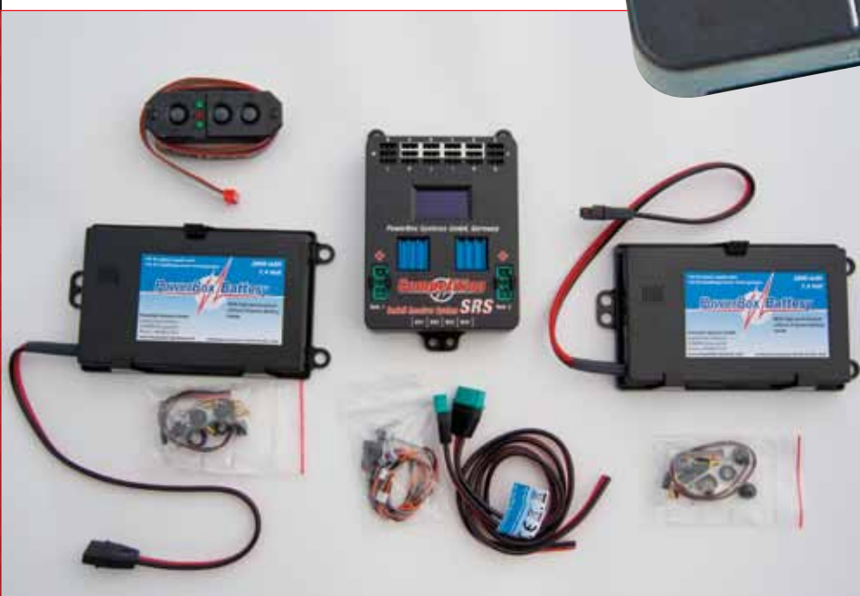
This is the package that I purchased. It includes two 2800-mAh 7.4-volt LiPo battery packs, a switch, cables and the Competition SRS power supply.
