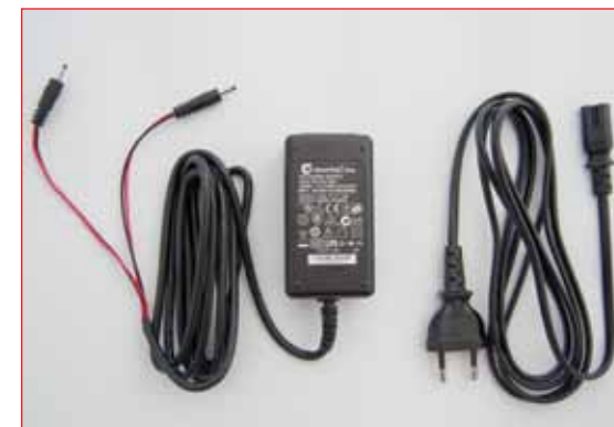
The 120/240 VAC wall charger is also designed to charge both PowerBox LiPo packs at the same time. Mine came with the plug used in Germany, which I changed out for a U.S. type.
