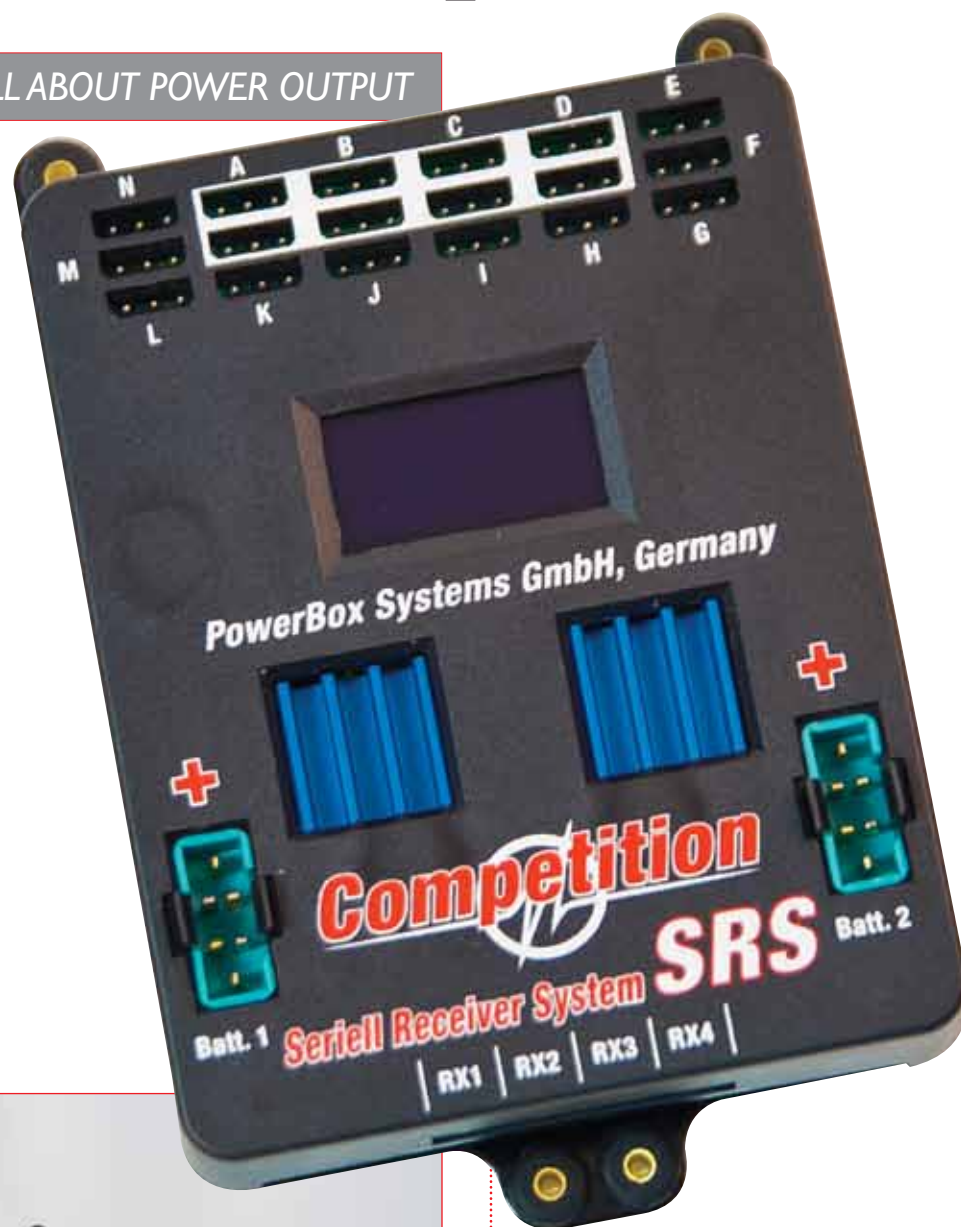
The new PowerBox Competition SRS includes inputs for two battery packs, heat sinks, four ports for remote receivers and a 128 x 64 OLED display.
