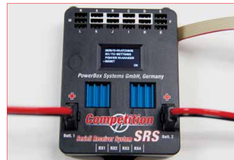
If you need to use your PowerBox Competition SRS in another model, you can reset all the program functions and parameters you've saved at this screen. Then you'll have it ready for reuse.
