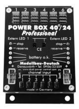
Featuring six servo-pulse amplifiers plus two independent voltage-controllers
