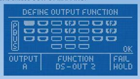
This menu displays a graphic image of the outputs. You can use the cursor to move through the outputs in order to select the one you wish to assign. Pressing the **SET button** at a selected output highlights the *FUNCTION* field, where you can select the signal to be assigned to this output. Pressing the **SET button** again highlights the *FAIL* field, and pressing the **SET button** a third time causes the cursor to move back to the Outputs field.
