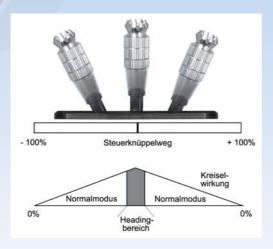
As can be seen from the diagram, gyro gain is suppressed proportionally with increasing stick travel. This reduces the tendency for the **iGyro** to counteract intentional control commands.
