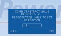
The undercarriage should now retract. If not, hold **button I** pressed in until the valve is triggered, and the undercarriage retracts. Press the **SET button** to move on to the next stage of the procedure.
