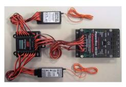
The photo below shows the method of connecting the system using a **PowerBox Evolution**. Seven channels of the Futaba G3 receiver are connected to the **RRS** module, plus the fail-safe channel. Since the **PowerBox Evolution** only caters for five remotely accessed channels, there are two vacant sockets on the **RRS** module to which two more servos can be connected. All the remaining channels of the Futaba G3 receiver could also be used directly at the receiver.
