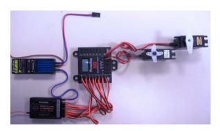
It makes no sense to connect one switch and one battery to each of the two receivers. In this configuration the batteries are not de-coupled, and could therefore discharge each other if one battery should fail.
