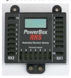
Sockets for seven patch leads from receiver 1 (RX 1)
