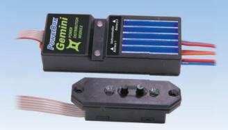
Double voltage stabilisation with linear regulation second voltage level for gyros and gyro servos, electronic safety switch (SensorSwitch Mini)
