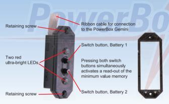
The pair of push-buttons is used to switch both power circuits on. This method of operation enables you to **check individually** each power circuit or battery.
