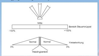
As can be seen from the diagrams above, gyro gain is suppressed progressively as control travel is increased. This reduces the effect of the **iGyro** in terms of counteracting the deliberate control command.
