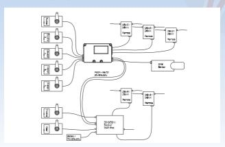
**Note:** if you wish to use a **PowerBox** (not **SRS**) as power supply with a Spektrum system, the unit is simply installed between the servos and the **iGyro**, or servos and receiver.
