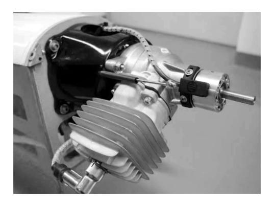
It is absolutely vital to ensure a tension free mounting of the engine. The surface that the engine is mounted on must be on an even plane (i.e., a flat and level surface) so that there is no strain on the engine itself. Again, this is a vital and critical requirement to avoid distorting the crank case, ruining the engine, and voiding your warranty.
