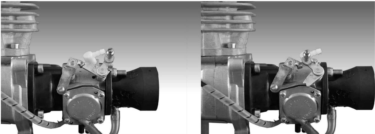
Note: The use of a soft pushrod for the throttle (plastic or nyrod) is not recommended. Use a metal or carbon fiber pushrod with a plastic ball joint or plastic clevis at each end. This will keep your RPM much more consistent and accurate around idle where it really counts.
