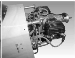
It is absolutely vital to ensure a tension free mounting of the engine. The surface that the engine is mounted on must be on an even plane (i.e., a flat and level surface) so that there is no strain on the engine itself. Again, this is a vital and critical requirement to avoid distorting the crank case, ruining the engine, and voiding your warranty.
