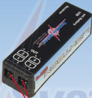
Outputs for the LEDs
